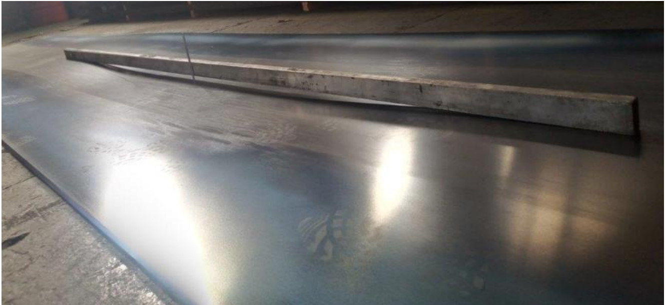
Figure 2 - Wavy central in hot-rolled steel plates or sheets and its measurement
