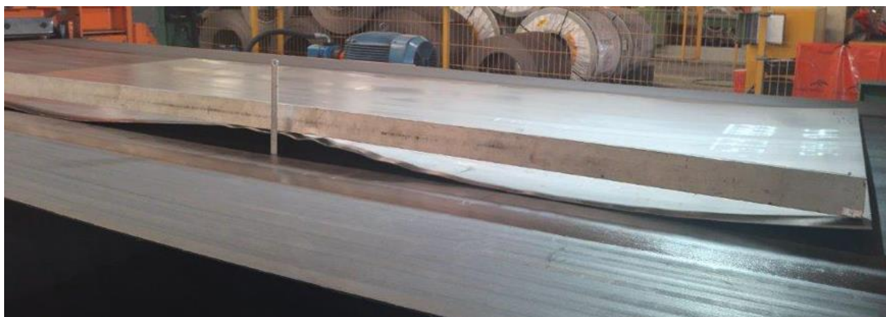
Figure 1 - Wavy edges in hot-rolled steel plates or sheets and its measurement
