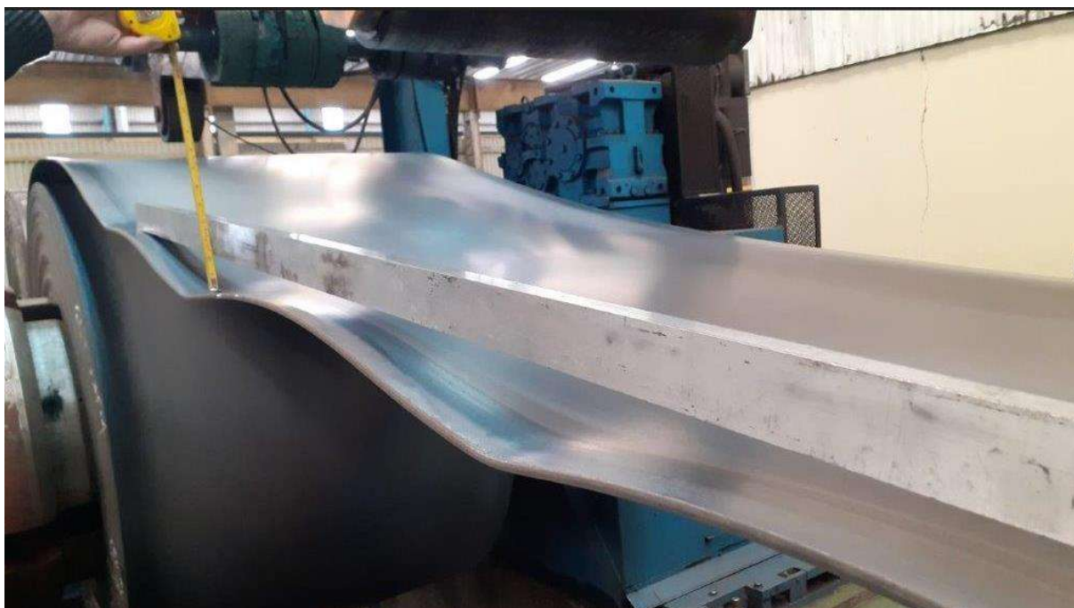
Figure 5 - Wavy edges in steel coils
