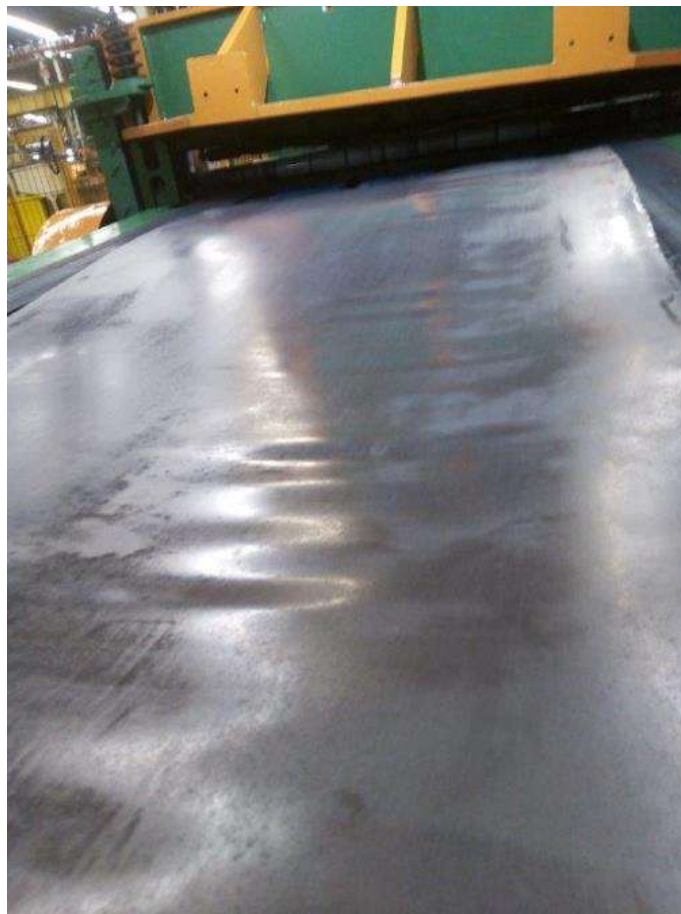
Figure 6 - Central buckles in steel coils
