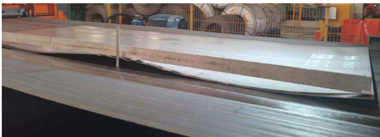
Figure 1 - Wavy edges in hot-rolled steel plates or sheets and its measurement
