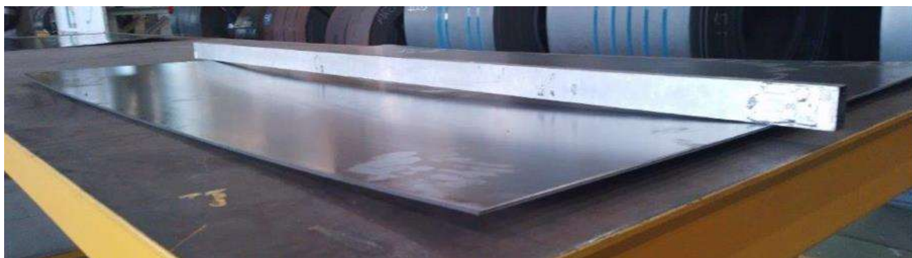
Figure 4 - Coil set in hot-rolled steel plates or sheets and its measurement
