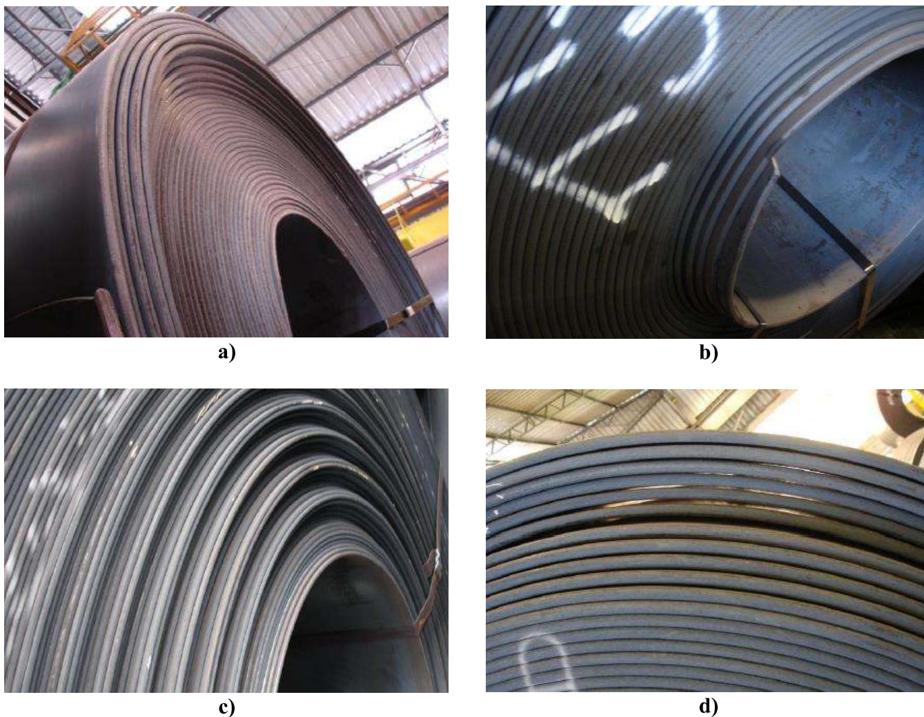
Figure 9 - Typical irregular winding problems not permitted. a) Telescope effect in the first outer turns; b) Telescope effect in the first inner turns; c) Irregular winding in all circumferential plane; and d) Loose winding
